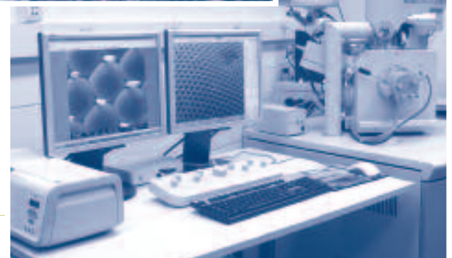
SEM FEI Quanta 200 FEG MKII scanning electron microscope
